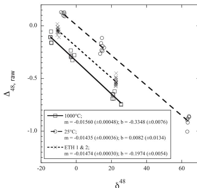
**Fig. 3.** Plot of  $\Delta_{48, \text{raw}}$  vs.  $\delta_{48}$  for  $\text{CO}_2$  equilibrated at 1000 °C and 25 °C, respectively, as well as for carbonate reference materials ETH 1 and ETH 2.  $\Delta_{48, \text{raw}}$  and  $\delta_{48}$  values are relative to the working gas composition. Slopes (m) and intercepts (b) of the corresponding linear regression lines, as well as their errors, are provided for further information.
