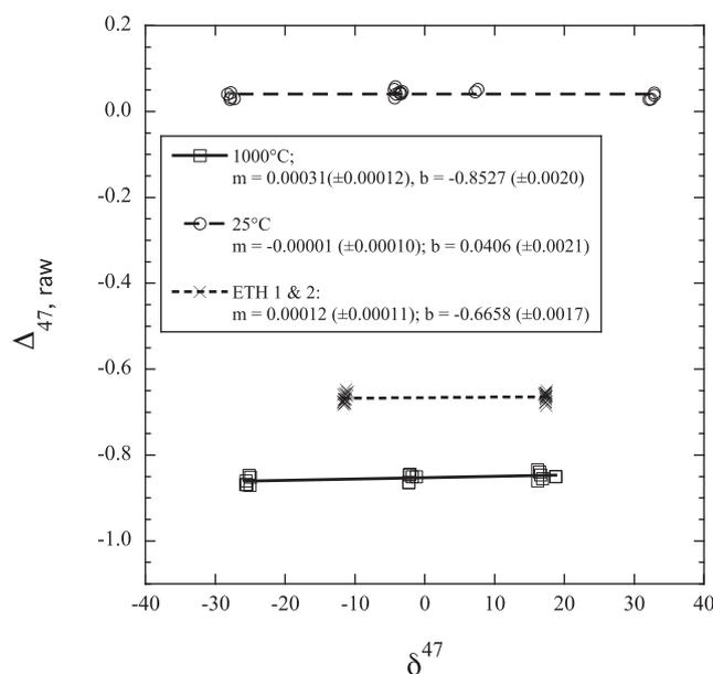
**Fig. 2.** Plot of  $\Delta_{47, \text{raw}}$  vs.  $\delta_{47}$  for  $\text{CO}_2$  equilibrated at 1000 °C and 25 °C, respectively, as well as for carbonate reference materials ETH 1 and ETH 2.  $\Delta_{47, \text{raw}}$  and  $\delta_{47}$  values are relative to the working gas composition. Slopes (m) and intercepts (b) of the corresponding regression lines, as well as their errors, are provided for further information.
