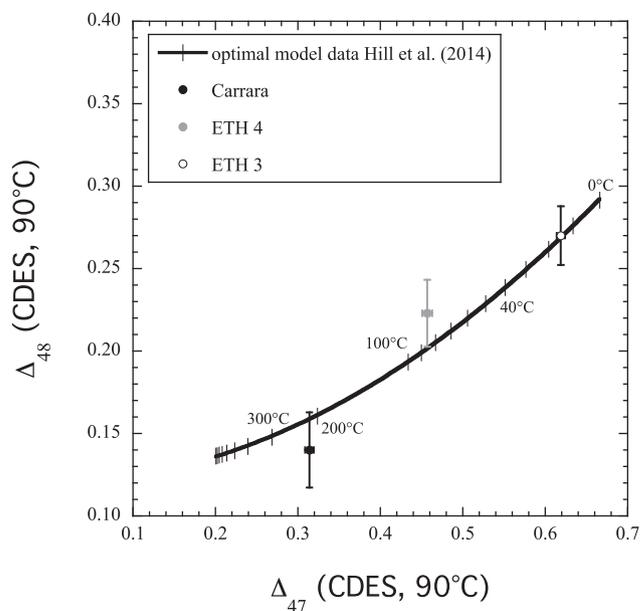
Fig. 4. Plot of  $\Delta_{48, \text{CDES } 90^\circ\text{C}}$  vs.  $\Delta_{47, \text{CDES } 90^\circ\text{C}}$  for ETH 3, ETH 4 and Carrara. Within errors (2 SE, 95 % confidence level), all data points agree with the theoretical equilibrium curve after adding the experimentally determined phosphoric acid fractionation factors of  $0.136 \text{‰}$  and  $0.196 \text{‰}$ , respectively, to the theoretical  $\Delta_{64}$  and  $\Delta_{63}$  values for calcite (Hill et al., 2014).
